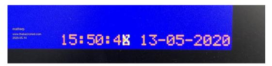
Note how the "X" appears to have overwritten the brown seconds units but the seconds are still incrementing underneath and pixels that are not covered by the "X" show normally.
