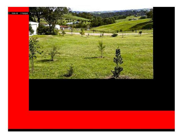
Time to load a 800 x 600 full colour jpg was 347 milliseconds. Worst case time to scroll the image with image wrap was 125 milliseconds. All other lower resolutions or lower colour depths will be faster.
